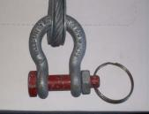
The screw pin shackle is capable of being used at full
